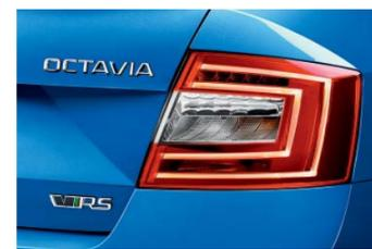
The **rear lights**, illumination of which creates a double C letter, are equipped with energy efficient **LED diodes**. (The photo shows the liftback version.)
