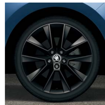
7.0J x 17" Savio alloy wheels in matt black design for tyre 215/40 R17
