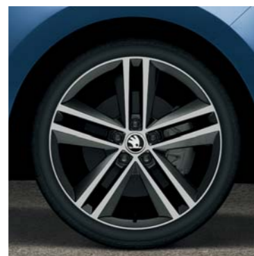
7.0J x 17" Ray alloy wheels in glossy black design for tyre 215/40 R17
